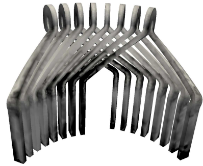
Figure 3: Total stress distribution issued from the mechanical resolution. High values are dark colored.
