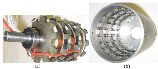
Fig. 1. Photo of the SMC TFM prototype: (a) stator; (b) rotor
