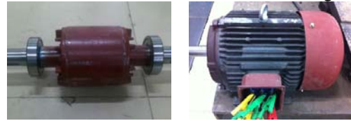
Fig.3 Improved non-skewed rotor and the prototype
