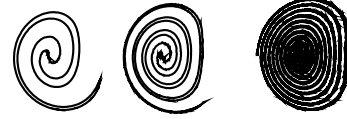
Figure 5: Blob of dye after (from left to right) 1, 2, and 5 periods with the rotating field and 2\pi/\omega = 2/3 T_m .
