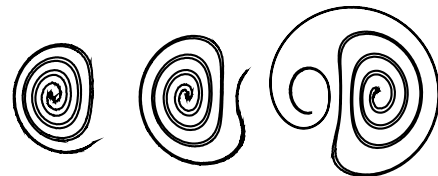
Figure 6: Comparison of blobs of dye at the same time between 2\pi/\omega = 2/3 T_m (left), 1/3 T_m (middle) and 2/9 T_m (right).
