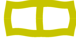
Figure 6: Deformation of the transformer at a chosen time in the period, 2 nd harmonic (100Hz).
