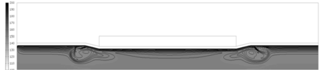
Fig. 5. Distribution of temperature T (in ^\circ\text{C} ) in melt for t = 0.4 \text{ s} (grey color – 150 ^\circ\text{C} , black color – 200 ^\circ\text{C} )
