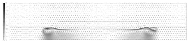
Fig. 6. Distribution of the module of velocity \mathbf{v} in melt for t = 0.4 \text{ s} (white color – 0 \text{ms}^{-1} , black color – 2 \text{ms}^{-1} )
