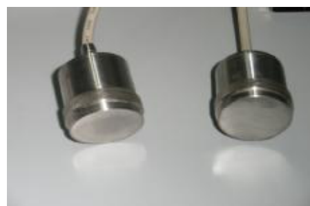
Fig.2 The model of 16-array elements ultrasonic phased array
