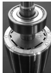
(a) Prototype of LSPMSM (b) Torque comparison of Experiment with FEM Fig. 4. Experiment results
