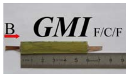
Fig. 1 : Sandwiched structure with Finemet® and copper foils (thicknesses 20 \mu\text{m} )
