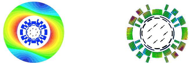
Fig. 2. Left: Cross-section through the nested MCBX corrector magnet. Right: Persistent-current magnetization due to a rotating field in the magnet aperture.
