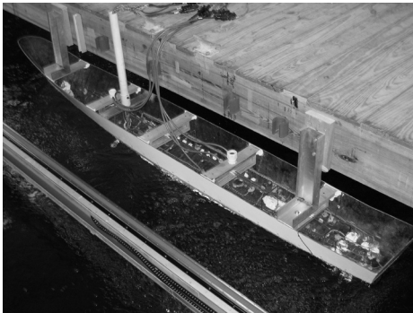
Fig. 1. 1/40 th mock-up set in measurement conditions
