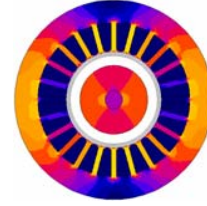
Fig. 1. 2D FEA model of high-speed motor with can
