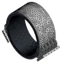
(a) FE model of BLDC motor stator
